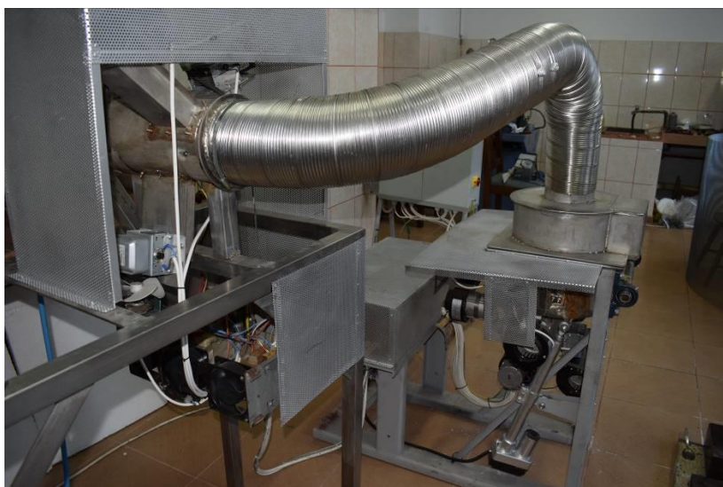
Fig. 3. Laboratory microwave furnace and gases thermal filter installation
