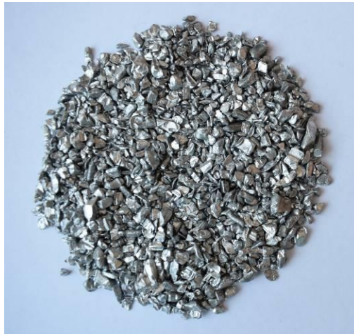
Fig. 1. Crushed aluminium cable waste
