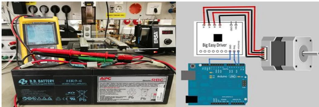
Fig. 4. Laboratory test bench and motor connection with driver and development board
