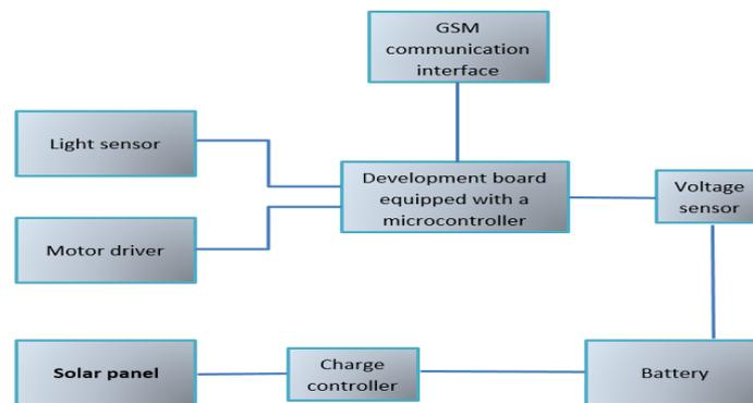
Fig. 3. Block diagram of the control system
