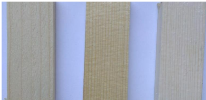
Fig. 2. The aspect of fir wood (from left to right: fir wood, fir wood + SEBS-MA; fir wood + SEBS-MA+ZnO)
