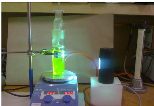
Fig. 3. *Photochemical reactor filled with the drug solution*
