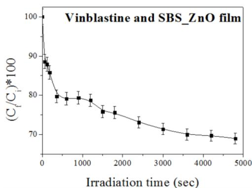
Fig. 5. Degradation of vinblastine in the presence of SBS\_ZnO film depending on the irradiation time
