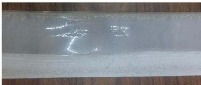
Fig. 2. SBS\_ZnO film obtained by spin casting
