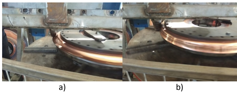
Fig. 4. The process of forming the outer flange of the lid of the fermentation column by the SR method: a) intermediate stage; b) the final stage
