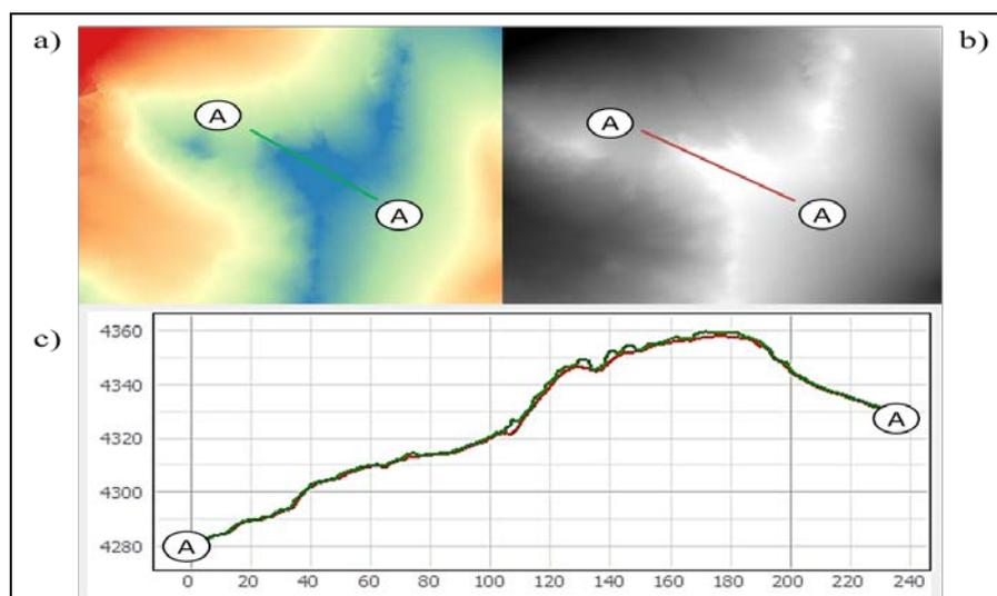
Fig. 6. Estimates of canopy height: a) - Digital Surface Model; b) - Digital Terrain Model; c) cut A - A indicating the differences in height (red = DEM heights, green = DSM heights)
