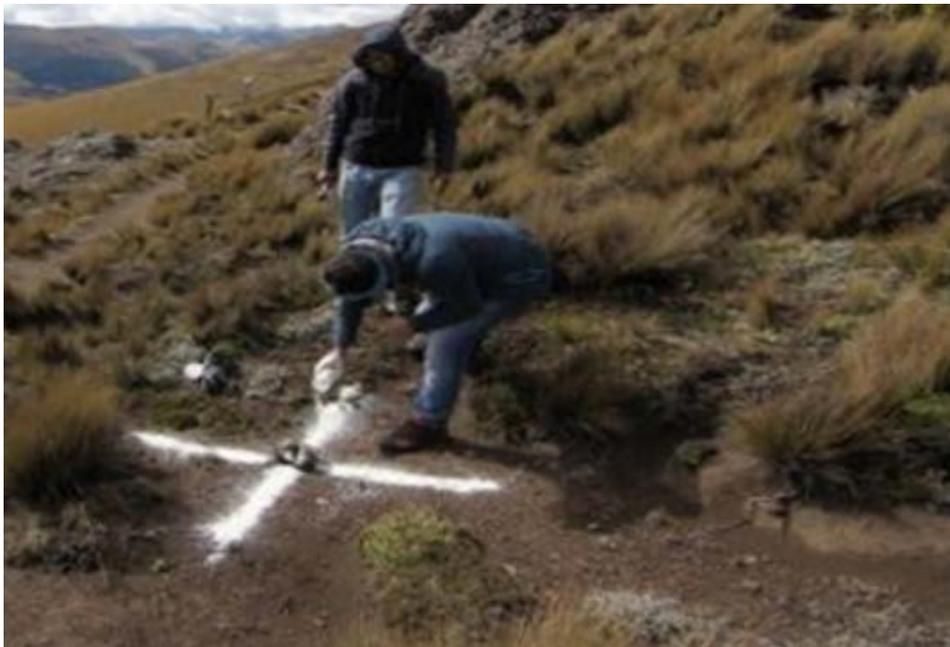
Fig. 2. *Field-marking of the GCPs*
