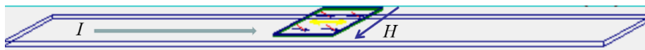
Fig. 3. The working principle of the GMR based current sensor. The red and blue arrows represent magnetizations from two adjacent magnetic layers.
