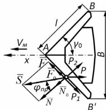
Fig. 2. Scheme of the passive cylindrical share
