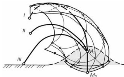
Fig. 1. Scheme of relative trajectory of motion heap particles along the share corresponding to curve I
