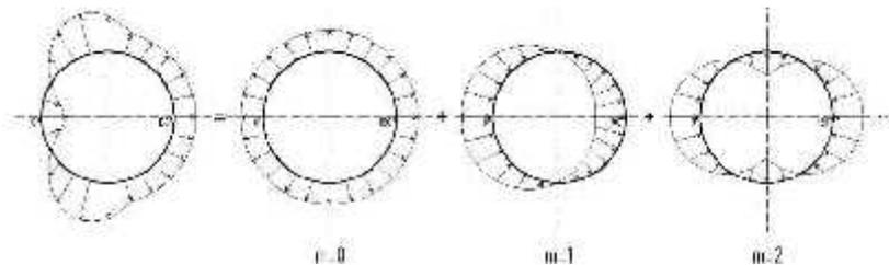
Fig. 1. *Distribution of wind load, on cylindrical mantle [8]*
