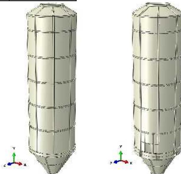
Fig. 5. 3D models of silo (left –model before remedation, right –after remedation)
