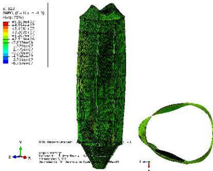
Fig. 9. *Deformations and stressess due to the effect of wind on the silo, for the model before remediation*
