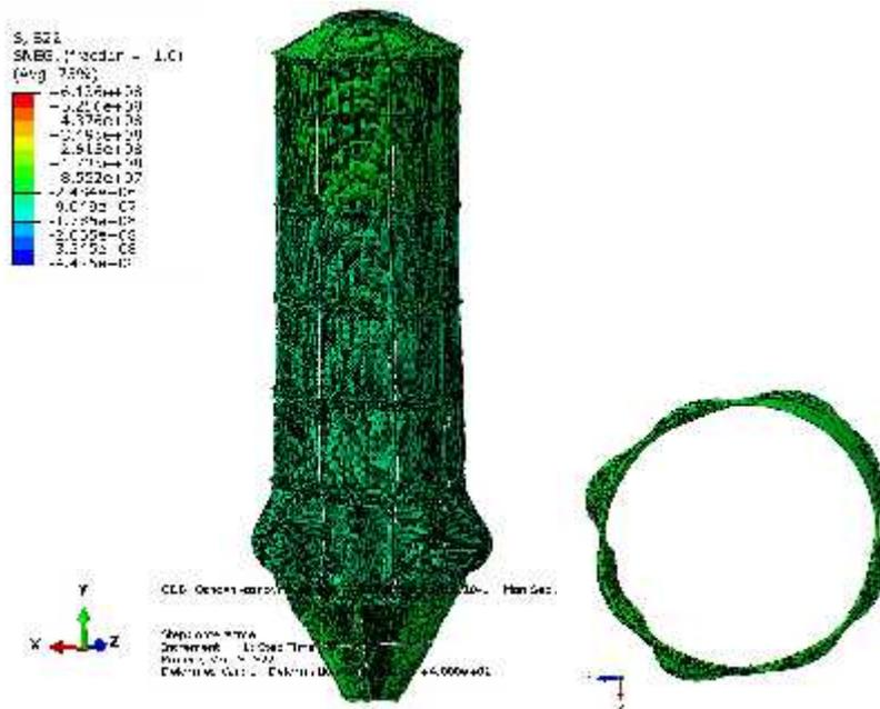
Fig. 6. Deformations and stresses due to their own load, for model before remediation
