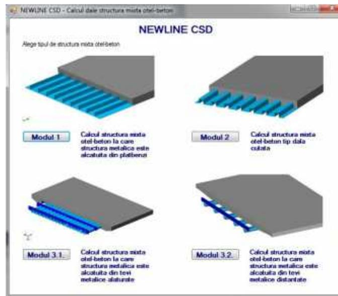
Fig. 6. Newline CSD (Composite Structure Design) bridge design program
