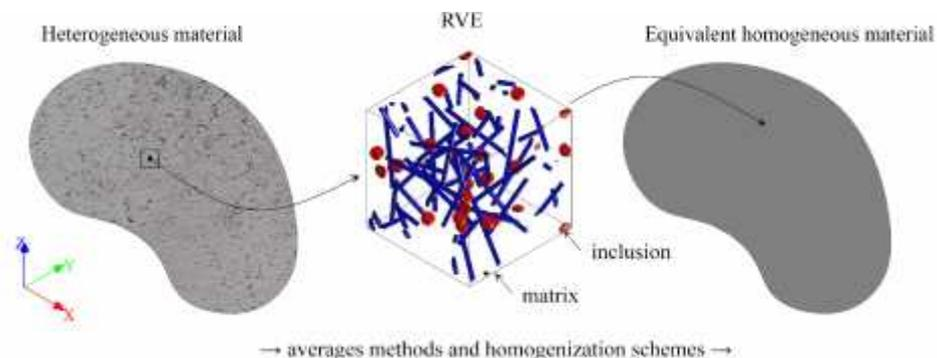
Fig. 3. Representation of the micro (meso) – macro transition through the RVE concept
