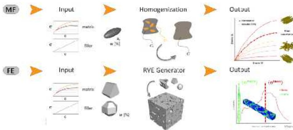
Fig. 2. Digimat-MF vs. Digimat-FE workflow overview
