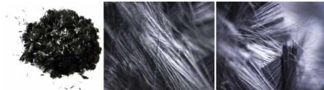
Fig. 1. *Chopped carbon fibres used in the research with 6 mm length. Normal and close-up (macro) photos.*
