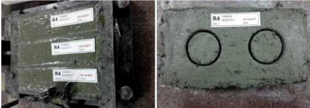
Fig. 2. The steel prism moulds (a) and the humidified full bricks with ~10 mm mortar layer used for test the adhesion of hardened mortar to the substrate (b).
