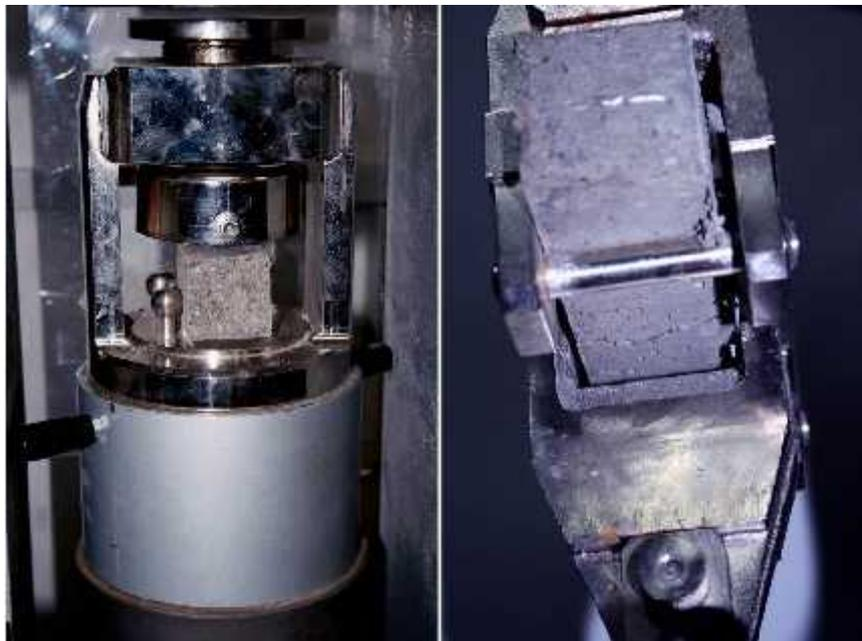
Fig. 3. Compression (a) and flexural strength test (b).
