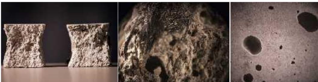
Fig. 4. *Failure modes of the specimens under the compression loading test and the materials (plain and CFRM) meso structure.*
