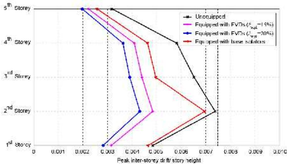
Fig. 5. Inter-storey drift/storey height profile, on the X direction of the structure, at SLS
