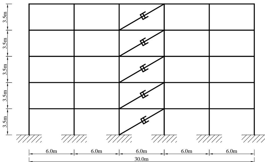
Fig. 2. Elevation view of a perimeter MRF equipped with dampers
