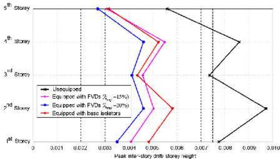
Fig. 6. Inter-storey drift/storey height profile, on the Y direction of the structure, at SLS
