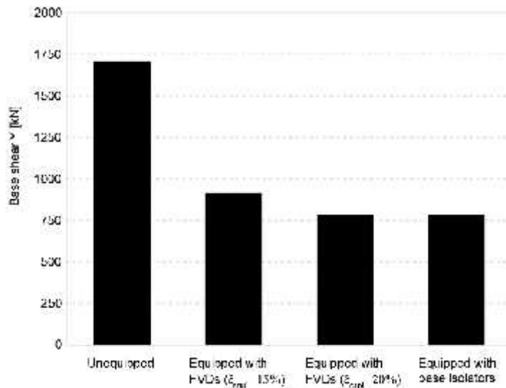
Fig. 4. Maximum base shears at ULS, on the Y direction of the structure
