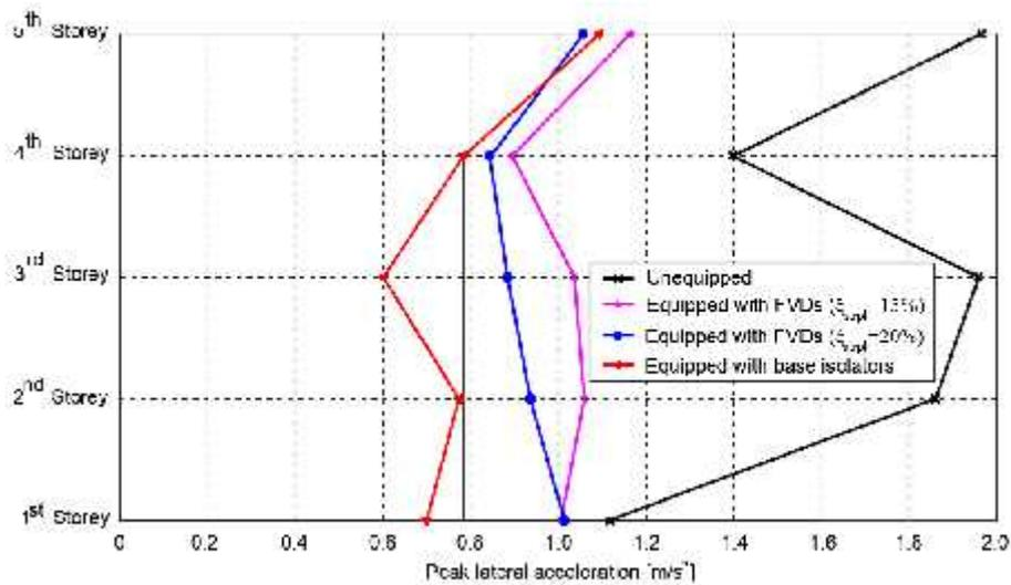
Fig. 8. Maximum storey accelerations profile, on the Y direction of the structure, at SLS
