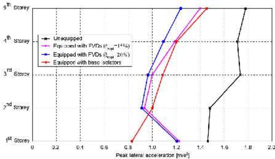
Fig. 7. Maximum storey accelerations profile, on the X direction of the structure, at SLS
