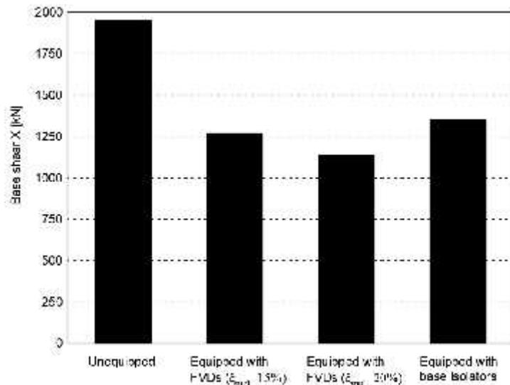
Fig. 3. Maximum base shears at ULS, on the X direction of the structure
