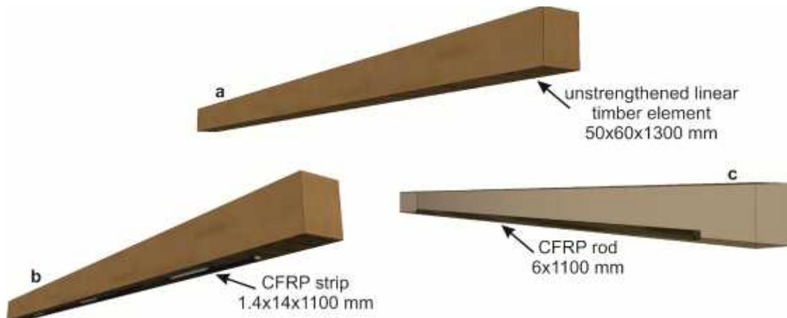
Fig. 2. *Assessed construction products. a. case study no. 1, b. case study no. 2, c. case study no. 3*
