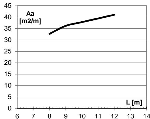
Fig. 6. Reinforcement - bridge span dependence
