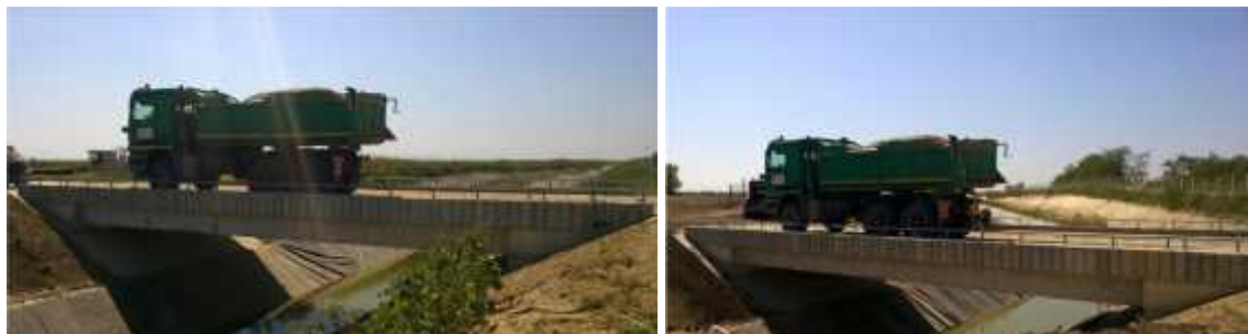
Fig. 3. Photo of the Bridge 1 and the Bridge 2 with trail load, longitudinal view
