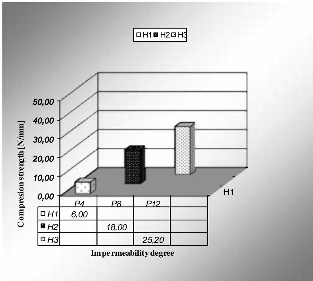
Fig.2. Variation of the permeability function of compression strength
