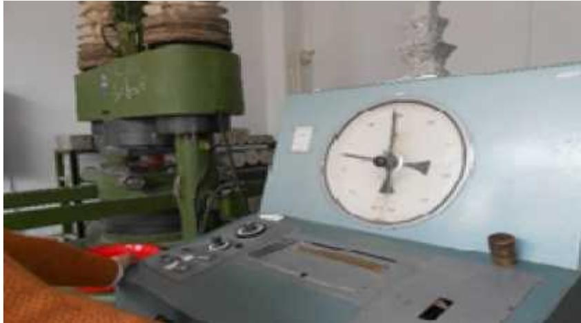
Fig. 5. *Determining the compressive strength*
