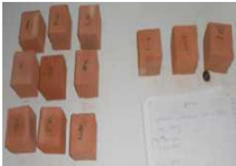
Fig. 1. *Array-samples extracted from masonry ceramic elements*
