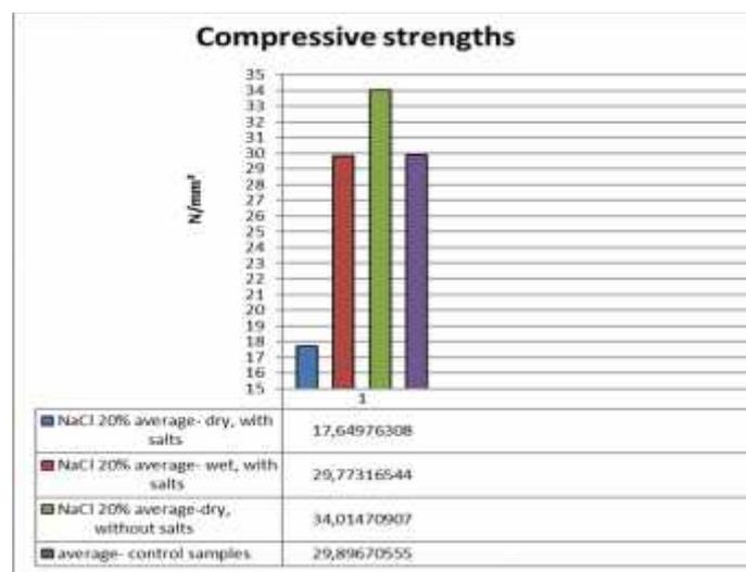
Fig. 7. Values obtained for the compressive strength of the tested array-samples
