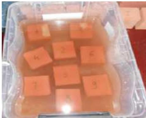
Fig. 3. *Array-samples in 20% concentration NaCl solution*
