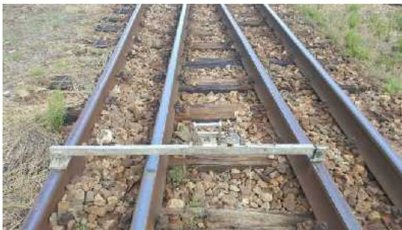
Fig. 5. *Gauge measurements at frog heel main rail*
