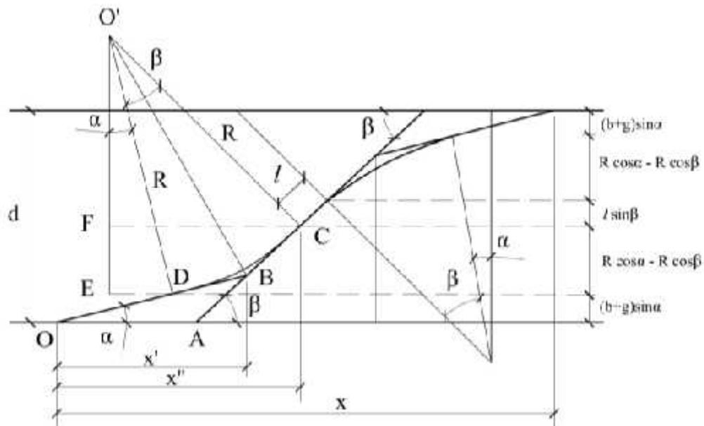
Fig. 3. Geometrical elements for turnouts
