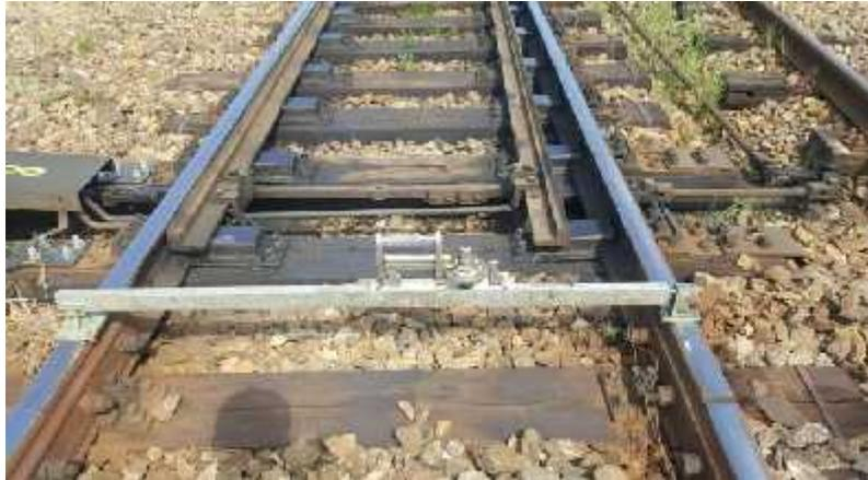
Fig. 4. *Gauge measurements at first joint*
