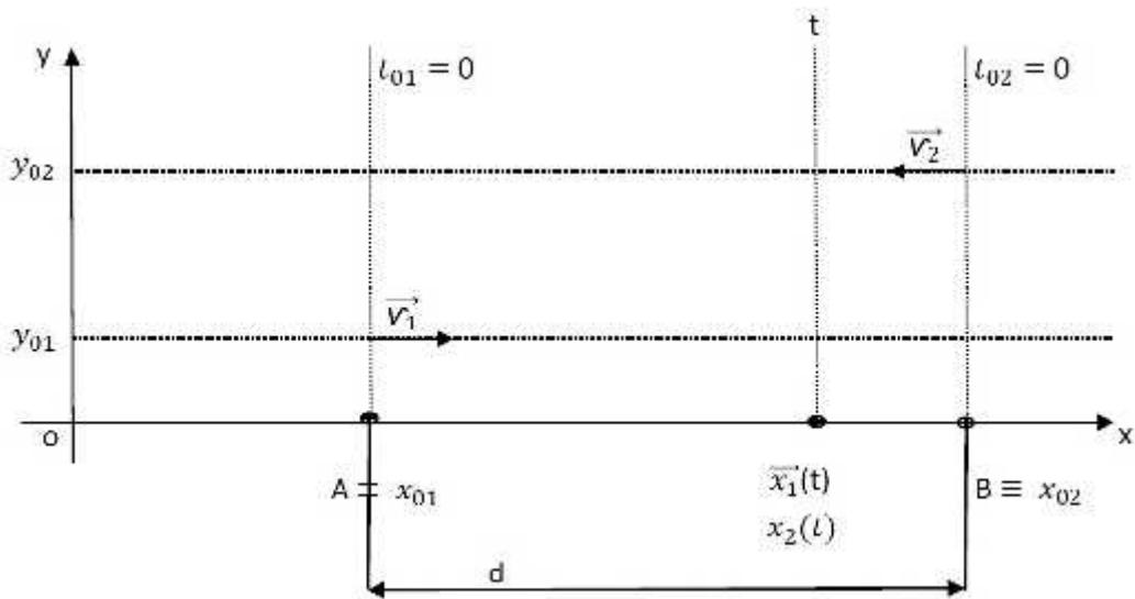
Fig. 4. *The diagram of the other two trains shipped in the opposite direction from the two stations*
