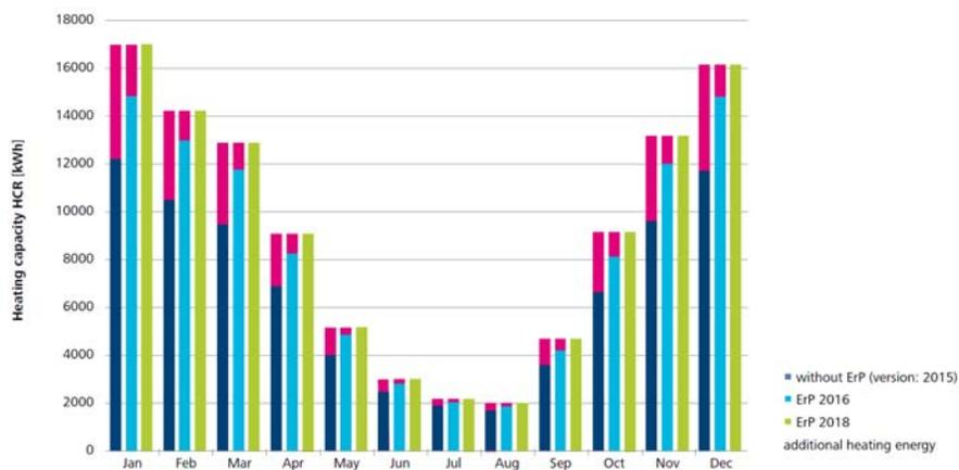
Fig. 1. Annual heating capacity HCR without Erp, with Erp 2016 and Erp 2018.
