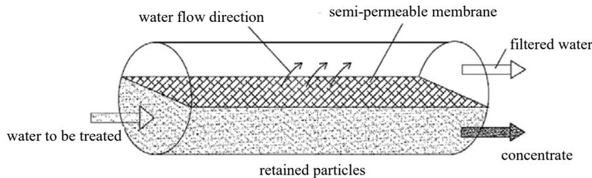
Fig. 2. Diagram representation of a membrane [3]
