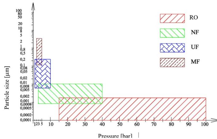
Fig. 3. Classification of baromembrane processes according to pressure and size of retained particles [1]
