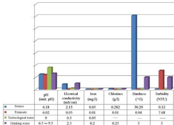
Fig. 5. Results for well water and system permeate in comparison to quality requirements for technological and drinking water [1]
