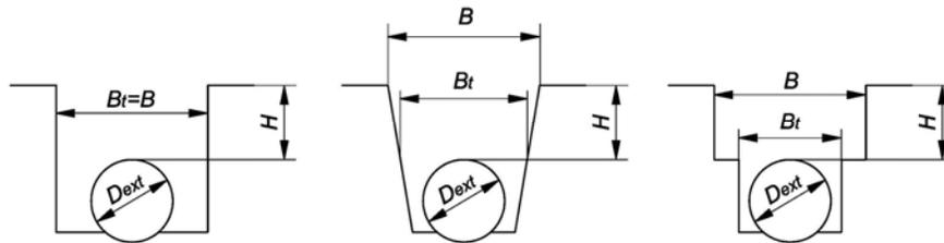
Fig. 5. Types of trenches used in sewer pipe laying [3]
