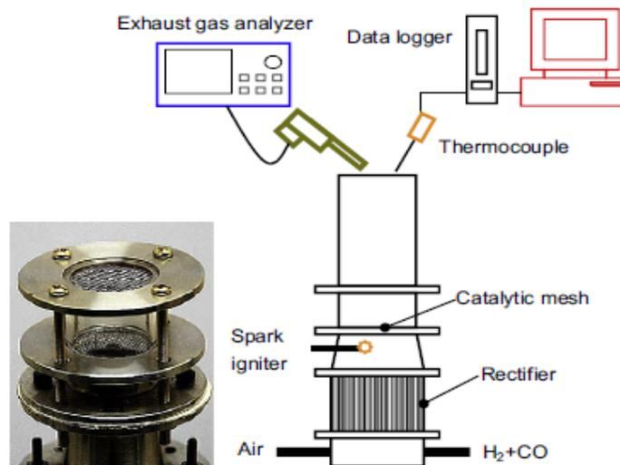
Fig. 2. Picture and scheme of the double-layer wire catalytic burner.
