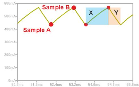
Fig. 2. Sample points and triangle approximation
