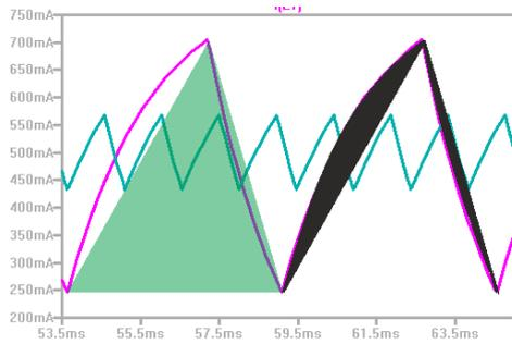
Fig. 1. Triangle waveform (green) and error area (black) at lower frequencies
