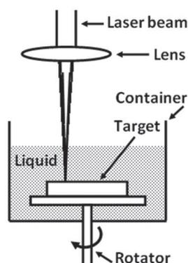
Fig. 3. *Experimental setup for nanoparticles synthesis by laser ablation in liquid* [13]
