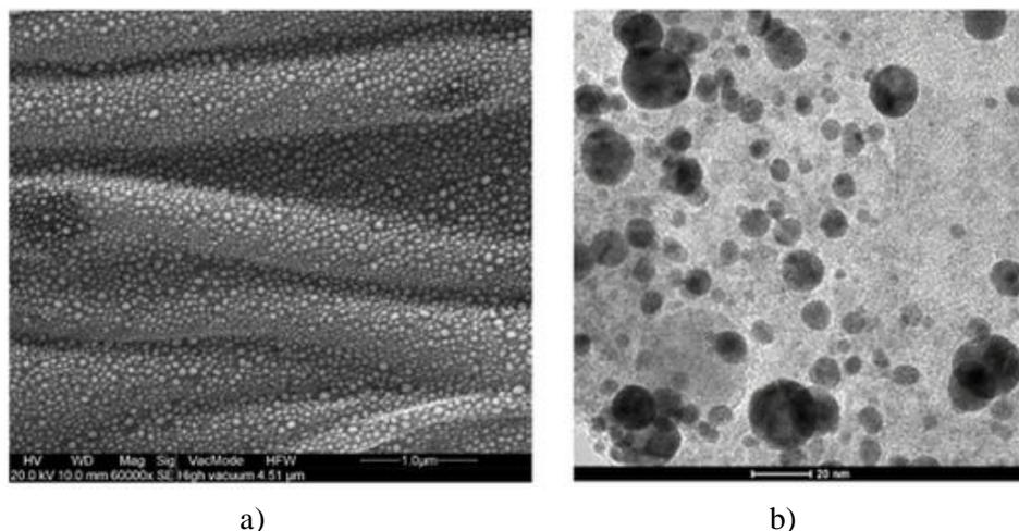
Fig. 6. SEM image of Ag NPs obtained after an irradiation time of 15 s (a); TEM images of Ag NPs collected after 30 s of irradiation (b) [2]
