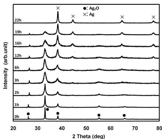
Fig. 5. XRD spectra of powder mixture milled as a function of milling time [8]
