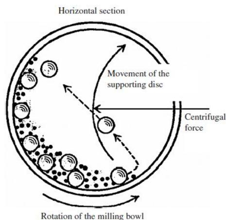
Fig. 2. *Schematic view of motion of the ball and powder mixture* [21]
