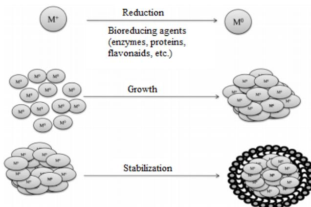
Fig. 4. Possible mechanisms of nanoparticle synthesis ( $M^+$ -metal ion) [10]
