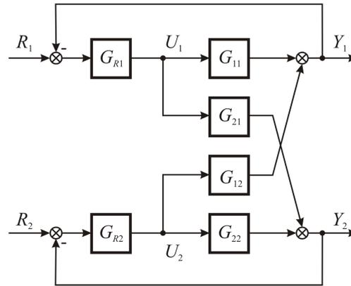
Fig. 1. Multi-input-multi-output control system
