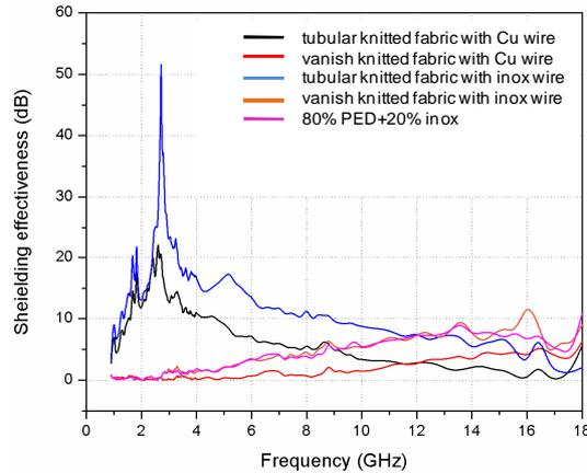
Fig. 2. *Shielding effectiveness versus frequency in domain 1-18 GHz for fibers with metal insertion*
