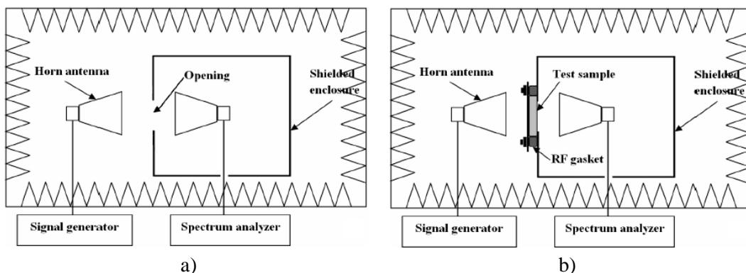
Fig. 1. *Experimental test: a) Reference measurement (without sample) and b) load measurement (with sample)*
