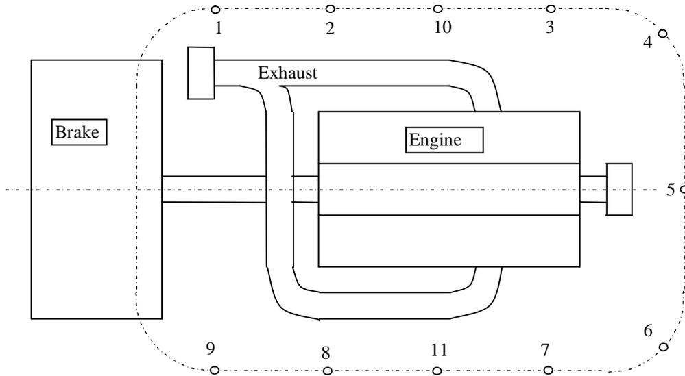
Fig. 4. *The configuration of noise measurement points*
