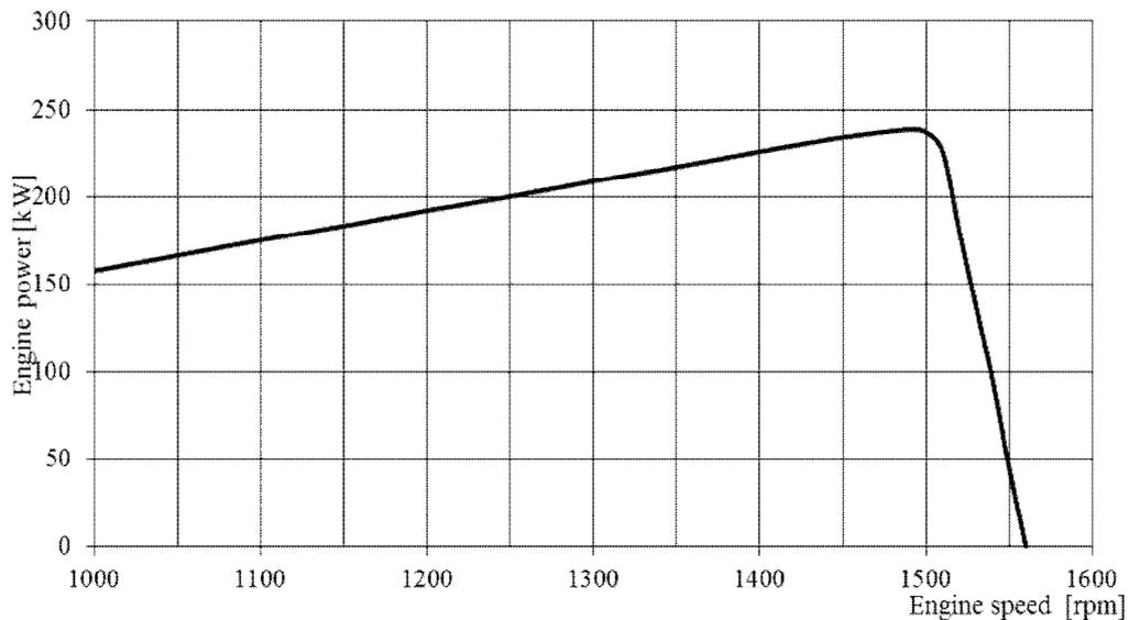
Fig. 1. Full load speed characteristic
