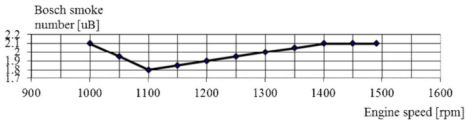
Fig. 5. *Smoke emission versus speed*
