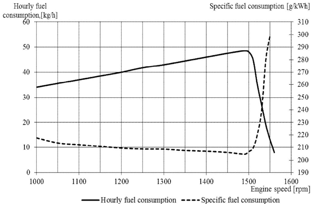
Fig. 2. *Hourly and specific fuel consumption versus speed*
