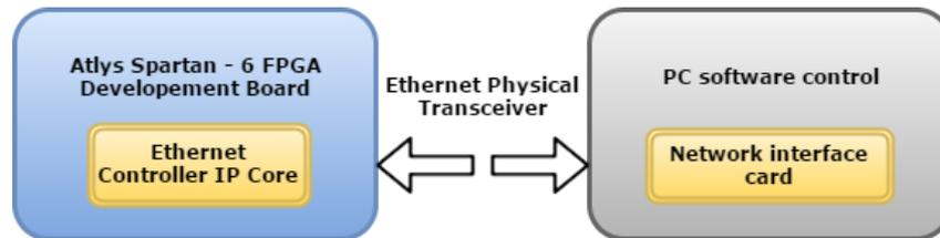
Fig. 2. *Communication FPGA-PC - general overview*
