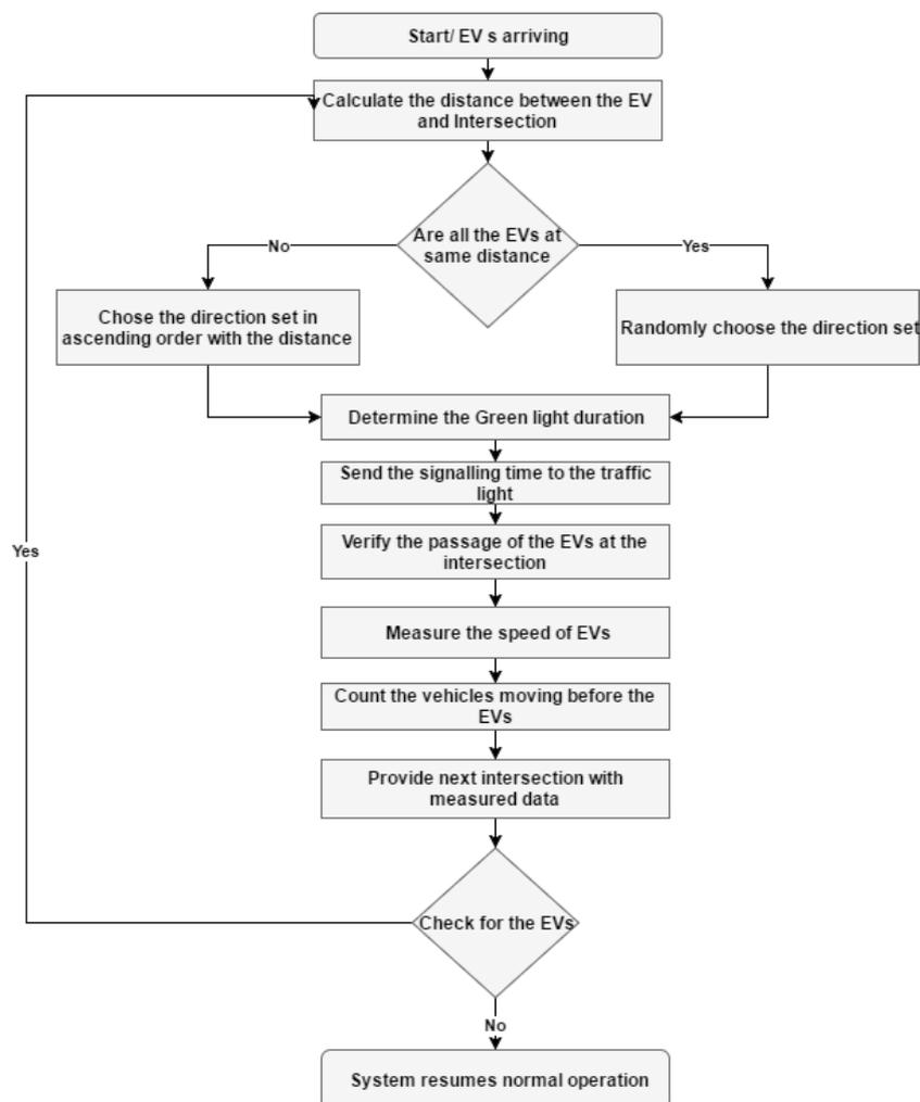
Fig. 3. *Distance-based emergency vehicle dispatching algorithm*
