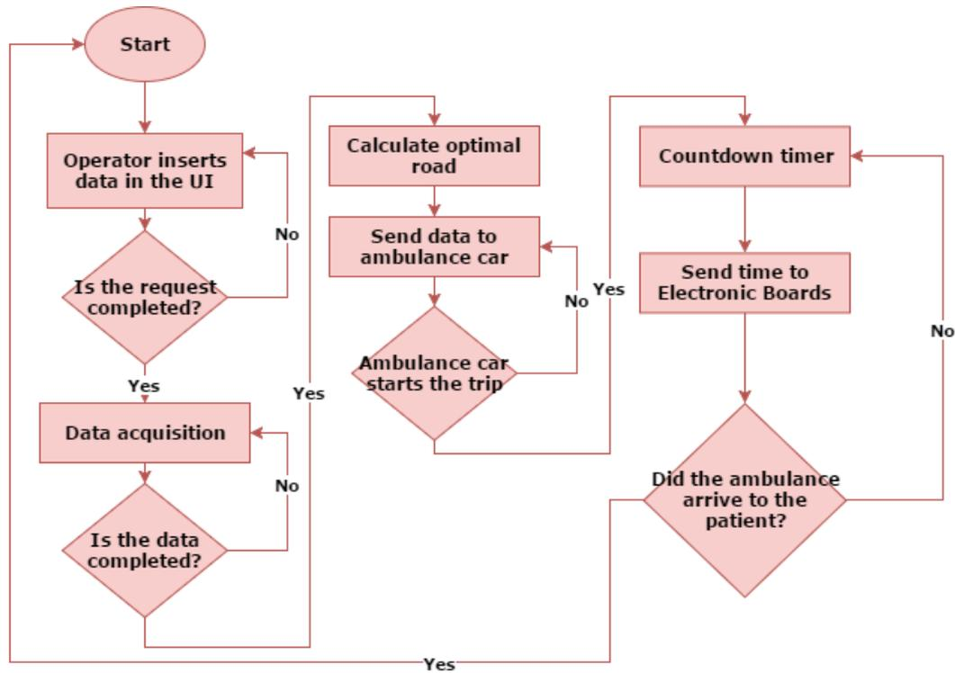
Fig. 4. *Flowchart of Software application*
