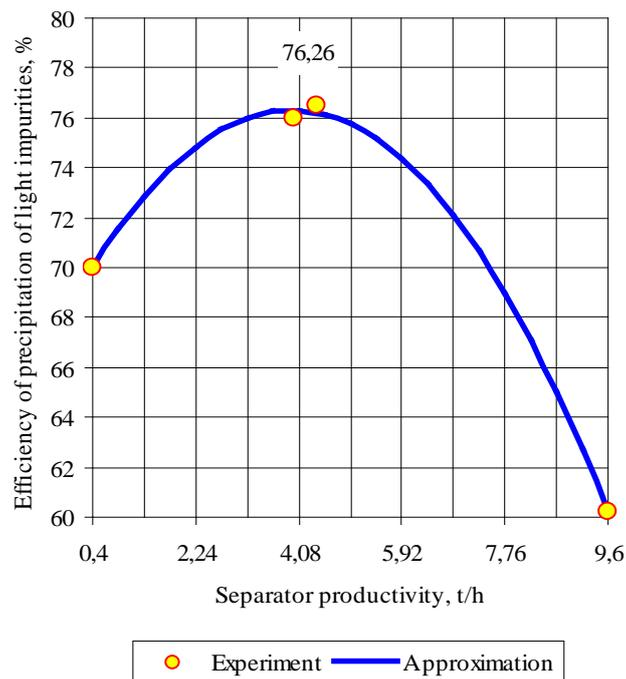
Fig. 8. Graph of the dependence of the technological efficiency of precipitation of light impurities  $E_k$ , % aspiration chamber of the flat-line separator on the efficiency of the separator  $q$
