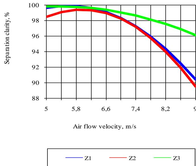
Fig. 5. Graphic dependencies of separation clarity  $Z$  on air flow velocity  $u$ : 1 – conical scatterer without blades; 2 – conical spreader with shoulder blades; 3 – serial spreader
