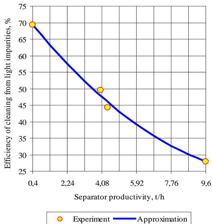
Fig. 7. Graph of the dependence of the technological efficiency of the air separation  $E$ , % of the modernized aspiration chamber on the performance of the separator  $q$
