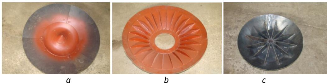
Fig. 1. *The general view of the spreaders, which carried out experimental research: a – conical scoop without blades; b – conical spreader with shoulder blades; c – serial spreader*
