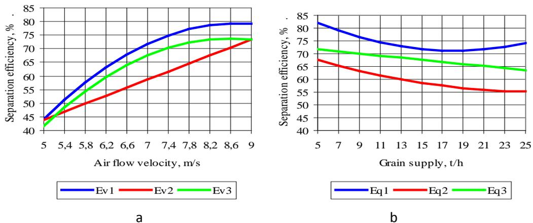
Fig. 4. *Graphic dependences of separation efficiency  $E$  on air flow velocity  $u$  (a) and grain supply  $q$  (b): 1 – conical scatterer without vanes; 2 – conical spreader with shoulder blades; 3 – serial spreader*
