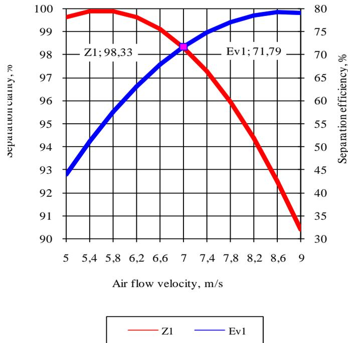
Fig. 6. Comparative graph of Z-resolution and separation efficiency E from the air flow velocity u for a conical scoop without blades
