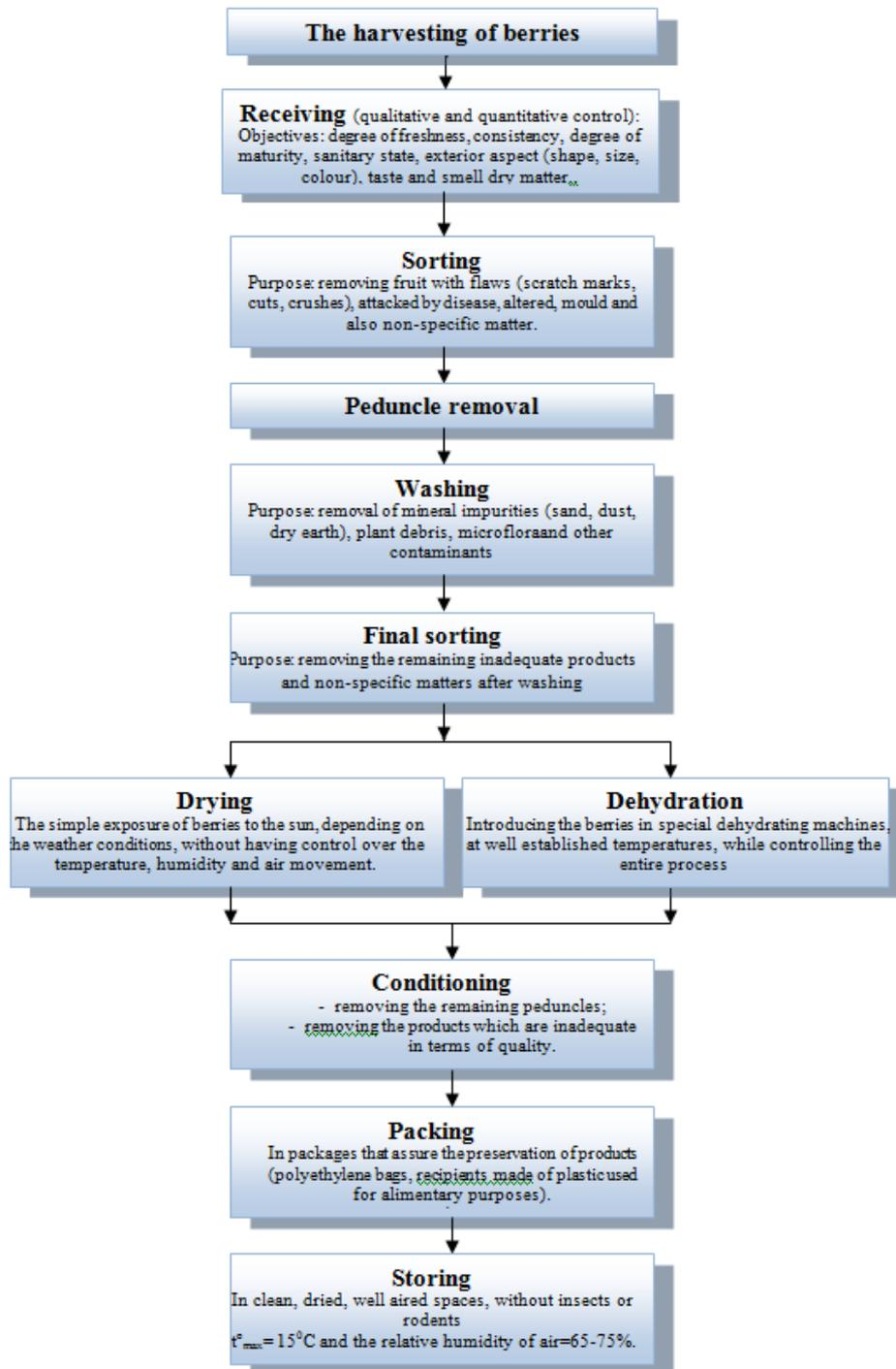
Fig.1. Technological figure of the drying/dehydration process of berries
