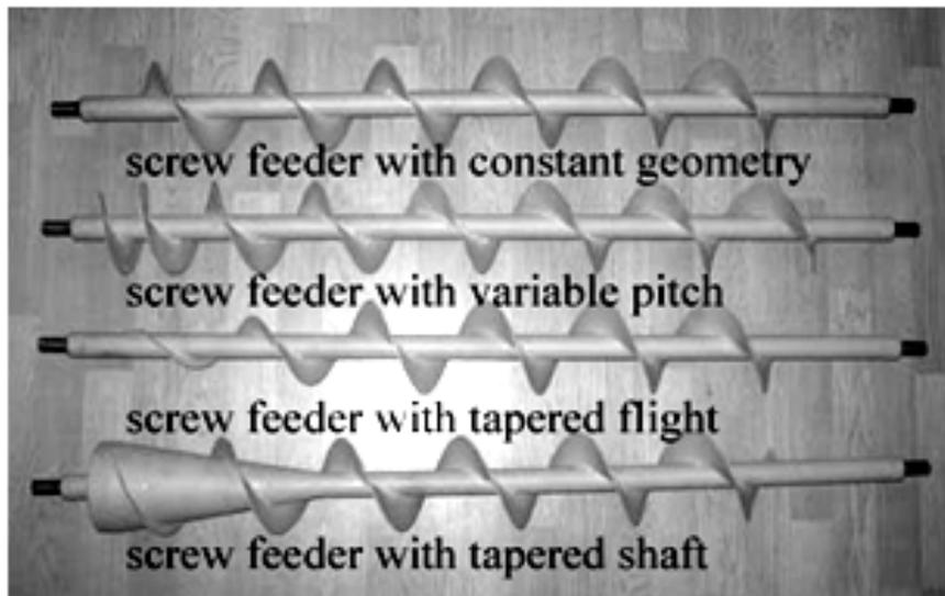
Fig. 4. *Interchangeable screw feeders with different extraction geometries*
