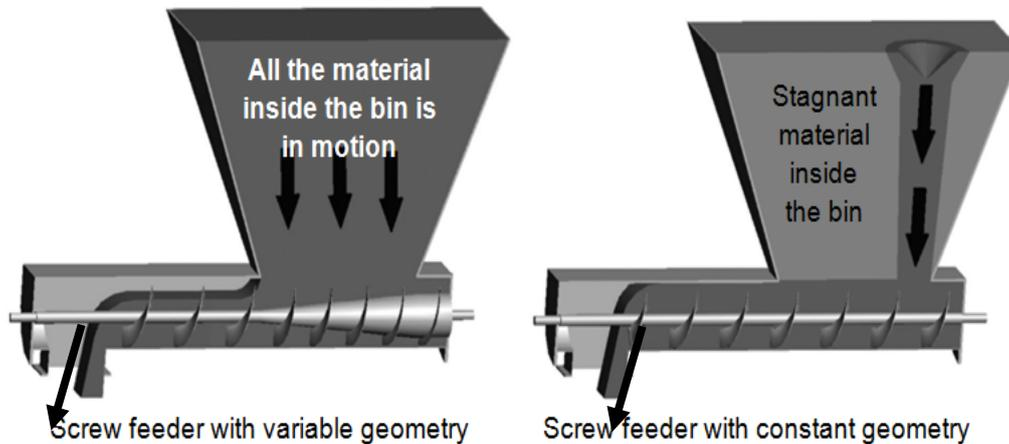
Fig. 1. Schematic presentation of material extraction with screw feeder with constant geometry right and variable geometry left [4]
