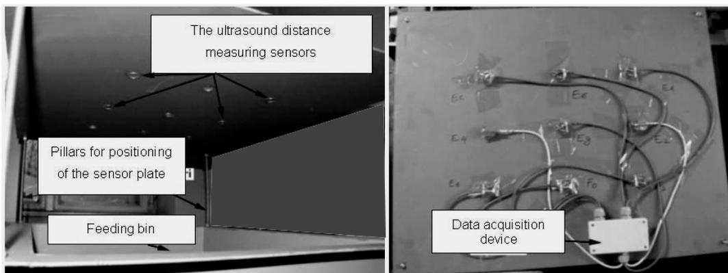
Fig. 5. *Sensor plate used to monitor the material level*
