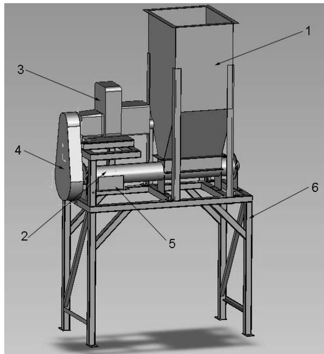
Fig. 3. 3D CAD modelling of the experimental stand used for the determination of the extraction flow profile of screw feeders. 1 – hopper; 2 – screw feeder chamber; 3 – power unit; 4 – chain transmission; 5 – screw feeder outlet; 6 – support frame
