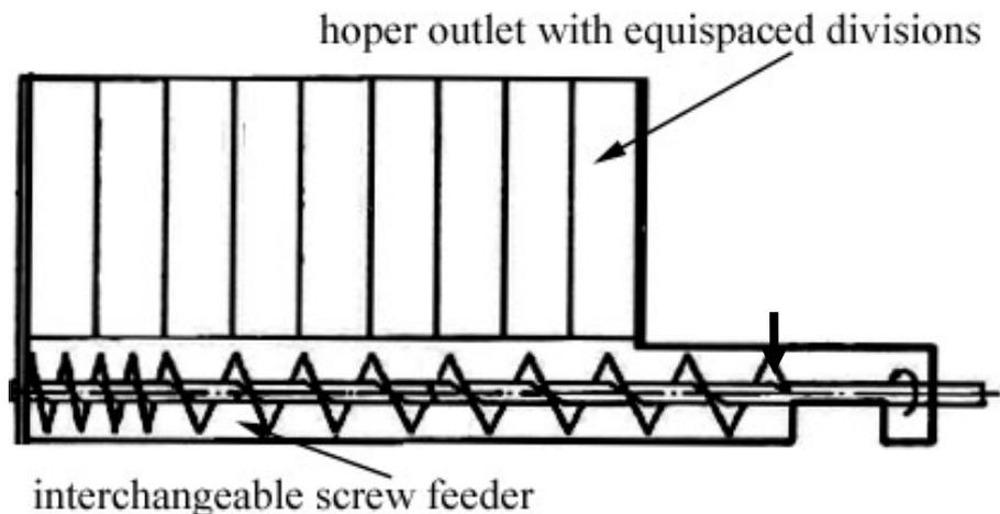
Fig. 2. Schematic representation of the experimental stand developed for studying of the flow profile of screw feeders [1]
