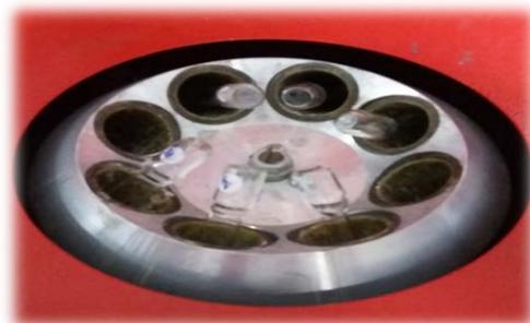
Fig. 17. Introducing the butyrometer in the centrifugal
