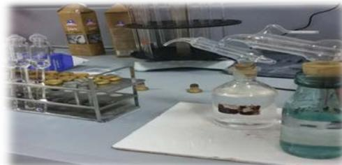
Fig. 11. *Gerber lactobutyrometer*
