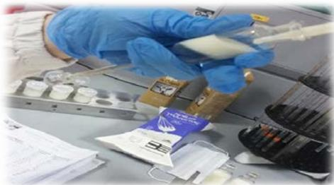
Fig. 14. Adding milk over the sulphuric acid
