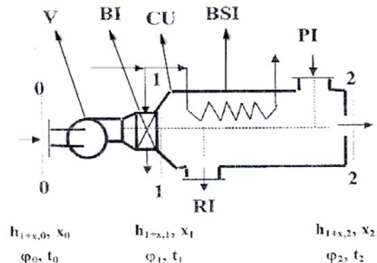
Fig. 1. Schematic diagram of the hot-air drying installation
