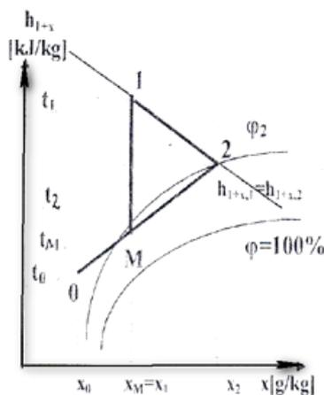
Fig. 3. Air-combustion gas mixing process, followed by the theoretical drying process [3]
