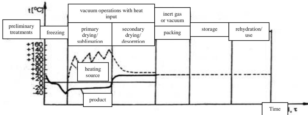
Fig. 2. Diagram of the lyophilization process
