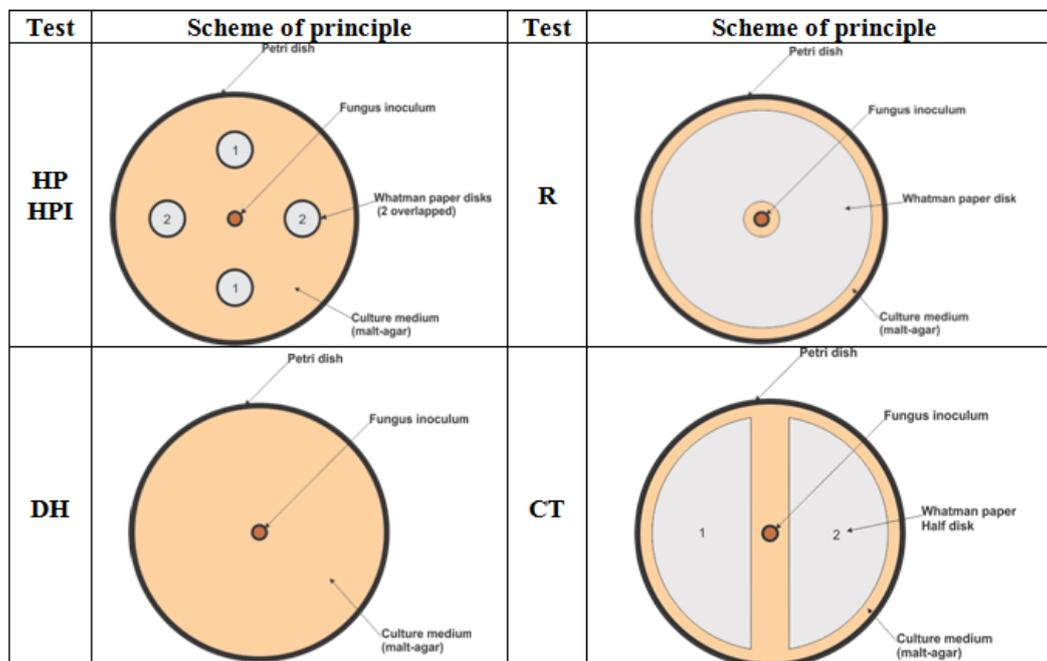
Fig.1. Schematic representation of the principles of the experimental screening tests
