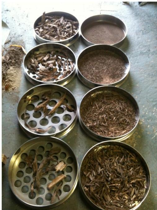
Fig. 1. Sieves used in fractioning out the particle sizes of the hogfuel
