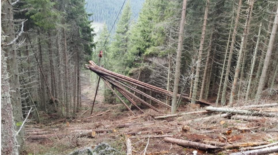
Fig. 1. A typical snapshot of yarding pre-bunched stems
