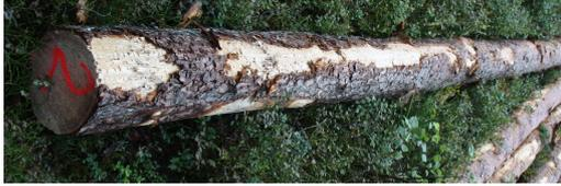
Fig. 2. An example of evaluation of the bark type according to bark presence on logs surface
