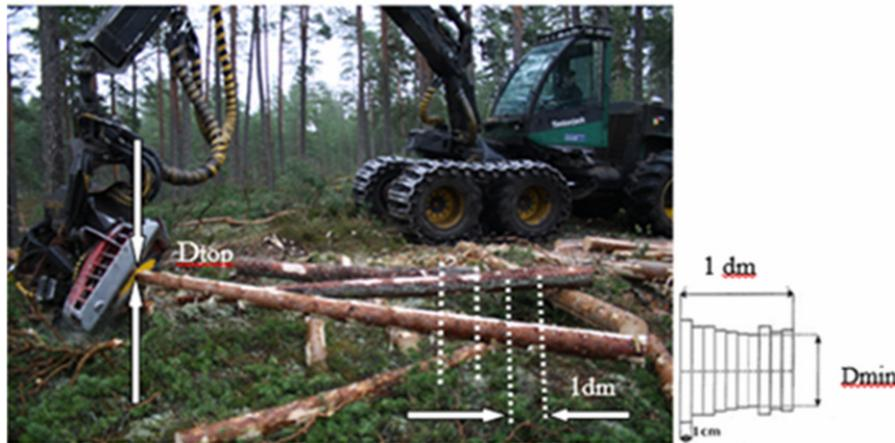
Fig. 1. Example of Timbermatic principles of controlling head diameter measuring, where  $D_{min} \geq D_{top}$
