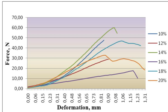
Fig. 2. *The influence of wheat grain moisture content on the shear grinding process*
