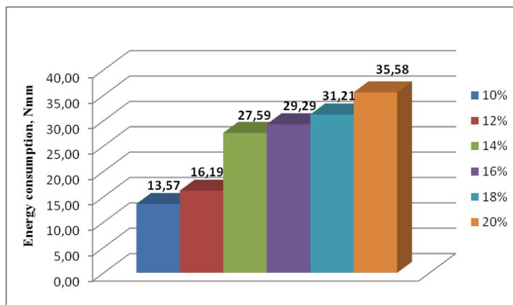
Fig. 3. *The evolution of energy consumption by shear grinding process on individual wheat grain at different values of moisture content*
