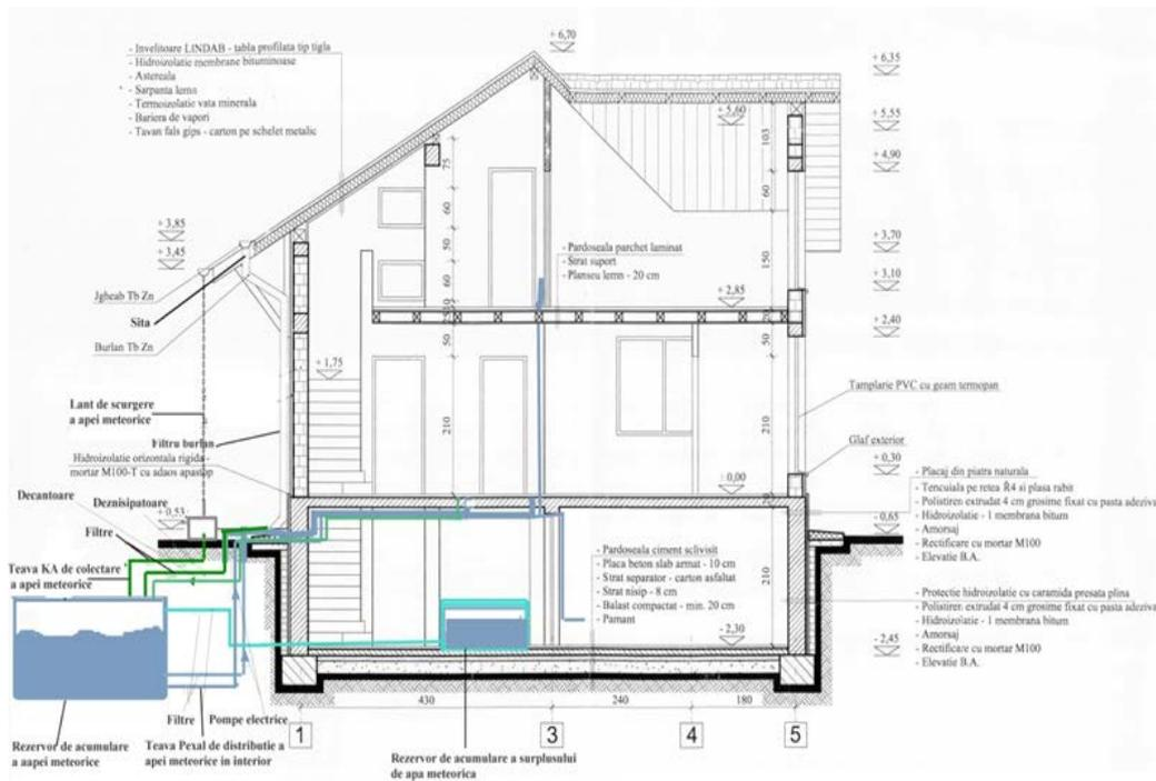
Fig. 3. Capture, storage, and distribution installation of rainwater for the accommodation unit
