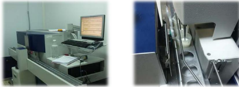
Fig. 3. The Fassomatic F.C. equipment used to count the somatic cells from the milk (NSC)
