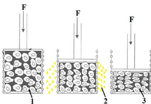
Fig. 1. Schematic representation of the pressing process (hydraulic presses):
