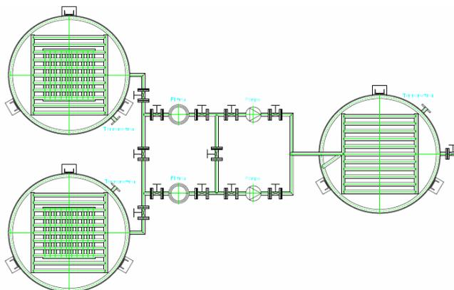
Fig. 5. *Schematic diagram of the paraffin emulsion preparation system at KASTAMONU, with two reactors and one stocking unit*
