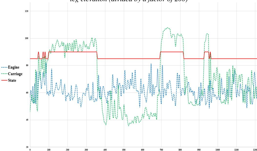
Fig. 5. A snapshot showing the carriage behaviour as interpreted by the algorithm for sound pressure level differentiation.
