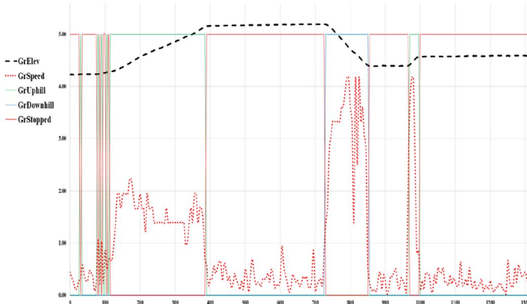
Fig. 4. A snapshot showing the carriage behaviour as interpreted by the algorithm against the variations in elevation and speed from the GPS data. Legend: red - stopped, green - uphill movement, blue - downhill movement, dotted red - leg speed, dotted black - leg elevation (divided by a factor of 200)
