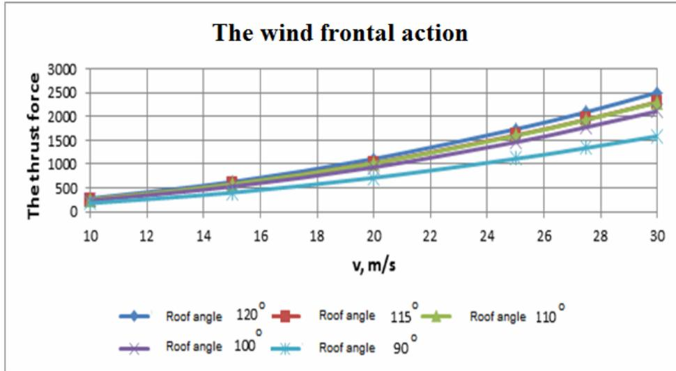
Fig. 4. The variation of the theoretically determined thrust force against the models to the wind frontal action with different speeds
