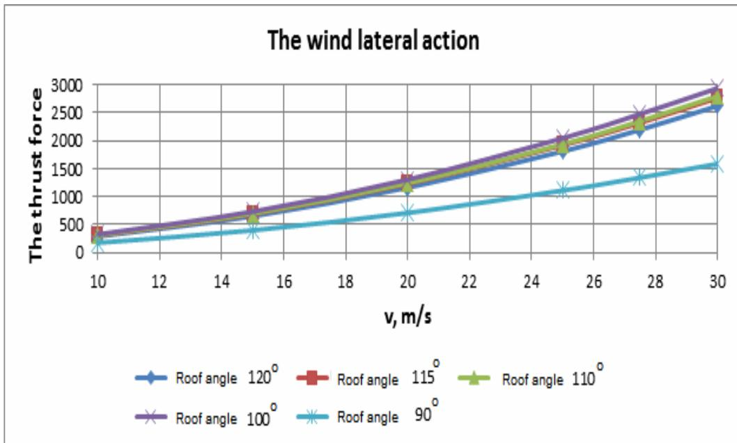
Fig. 6. The variation of the theoretically determined thrust force, exerted on the models to the wind lateral action with different speeds
