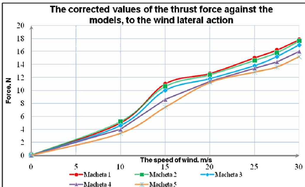
Fig. 7. The variations of the thrust forces exerted on the models to the wind lateral action, obtained as a result of the experimental research in the aerodynamic tunnel
