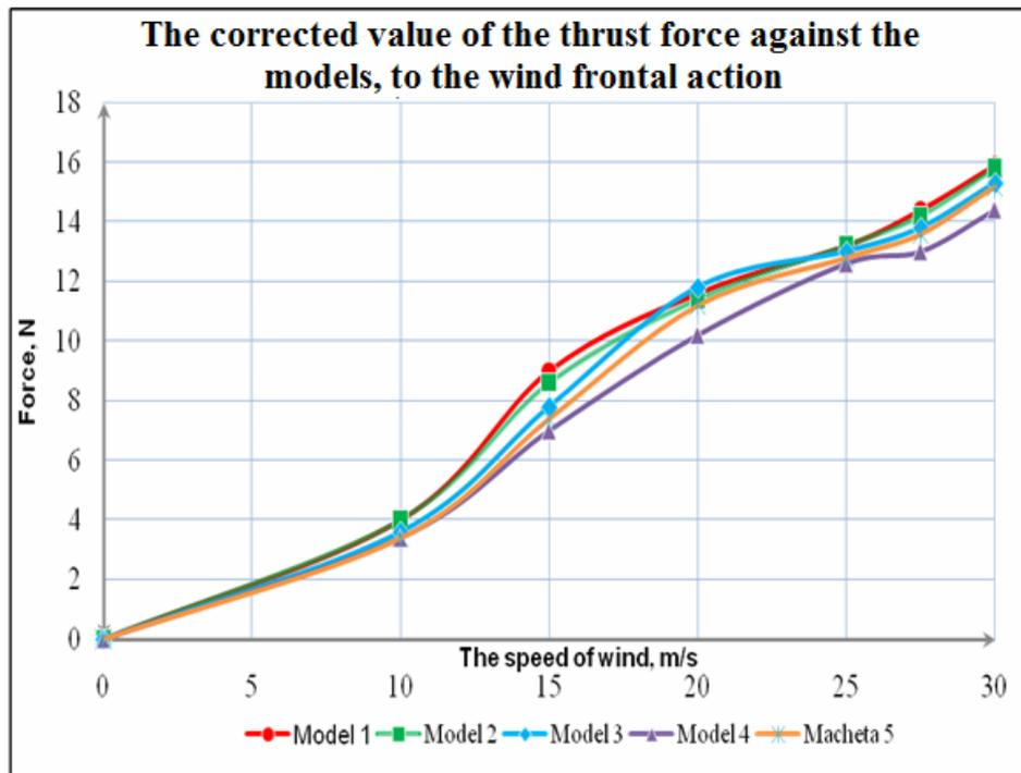
Fig. 5. The variation of the thrust forces, exerted on the models to the wind frontal action, obtained as a result of the experimental research in the aerodynamic tunnel
