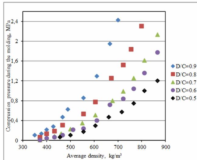
Fig. 3. The influence of compression pressure during the moulding of wood-cement mixture on the average density of the material at various ratios  $D/C$
