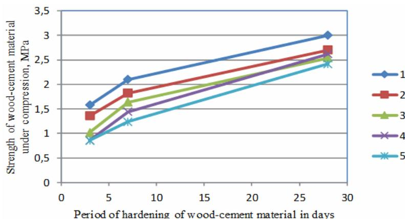
Fig. 1. *The dependence of the strength of wood-cement composite at various stages of hardening of the composition of wood fractured particles:*
