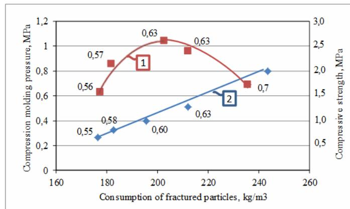
Fig. 4. The influence of the compression moulding pressure, consumption of fractured particles and the value  $D/C$  (the value of  $D/C$  is indicated by numbers) on the strength of arbolite at cement consumption at  $330 \text{ kg/m}^3$  [9]: 1 – compressive strength; 2 – compression moulding pressure
