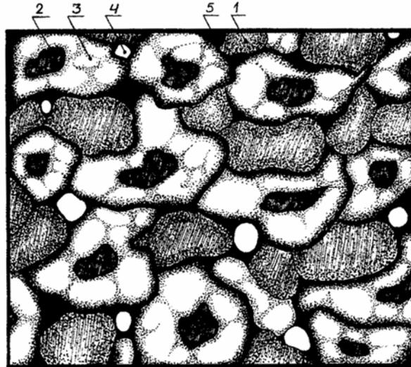
Fig. 2. *The scheme of the microstructure of system: wood filler - cement binder – water: 1 is wood filler; 2 are cement particles; 3 is shell of gel, formed from dissolved cement particles; 4 are air pores; 5 is free water.*
