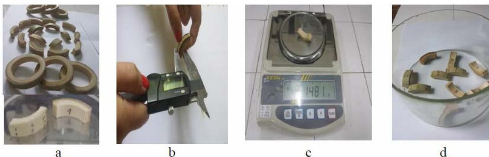
Fig. 5. *Sequences of water immersion test (a. – codification, b. – measuring, c. – weighing, d. – immersion)*
