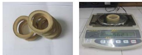
Fig. 3. *Samples for moisture content test*
