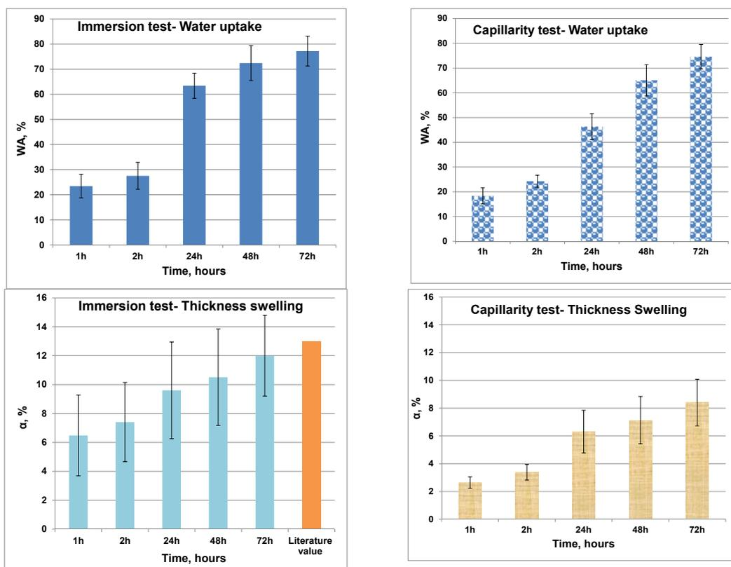
Fig. 9. Results after water immersion and capillarity test (water uptake and swelling)
