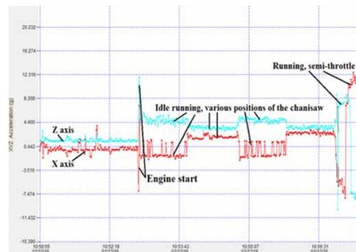
Fig. 2. *Patterns recorded by a vibration sensor for different regimes of engine functioning in the case of a chainsaw*
